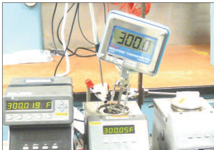
Wahl DST600 Series thermometer system being tested in the calibration lab of a major food processor, against two certified references.
