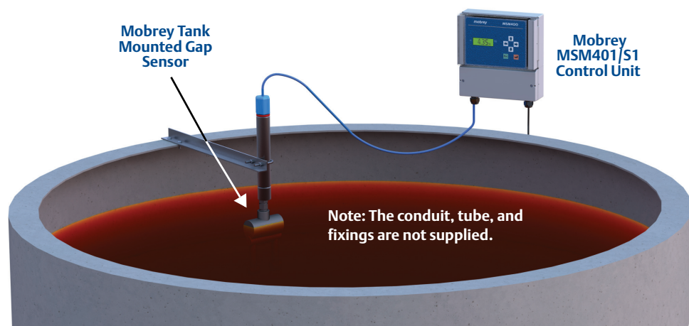
Figure 3-1. Mobrey Tank Mounted Gap Sensor
