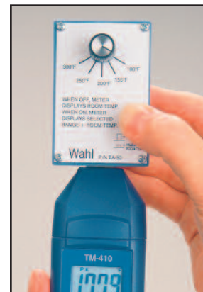
TM410 shown in use with NIST Certified TA50AFK Calibrator, page 10.
